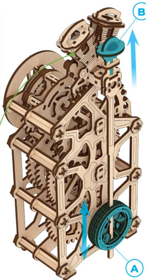
**ENG** It would be better to adjust the accuracy of the stroke at the middle spring rate. For adjustment, move the wheel weight (A) up (speed up) or down (slow down); if necessary, move the metal ball weight (B) up to slow down the clock further.
