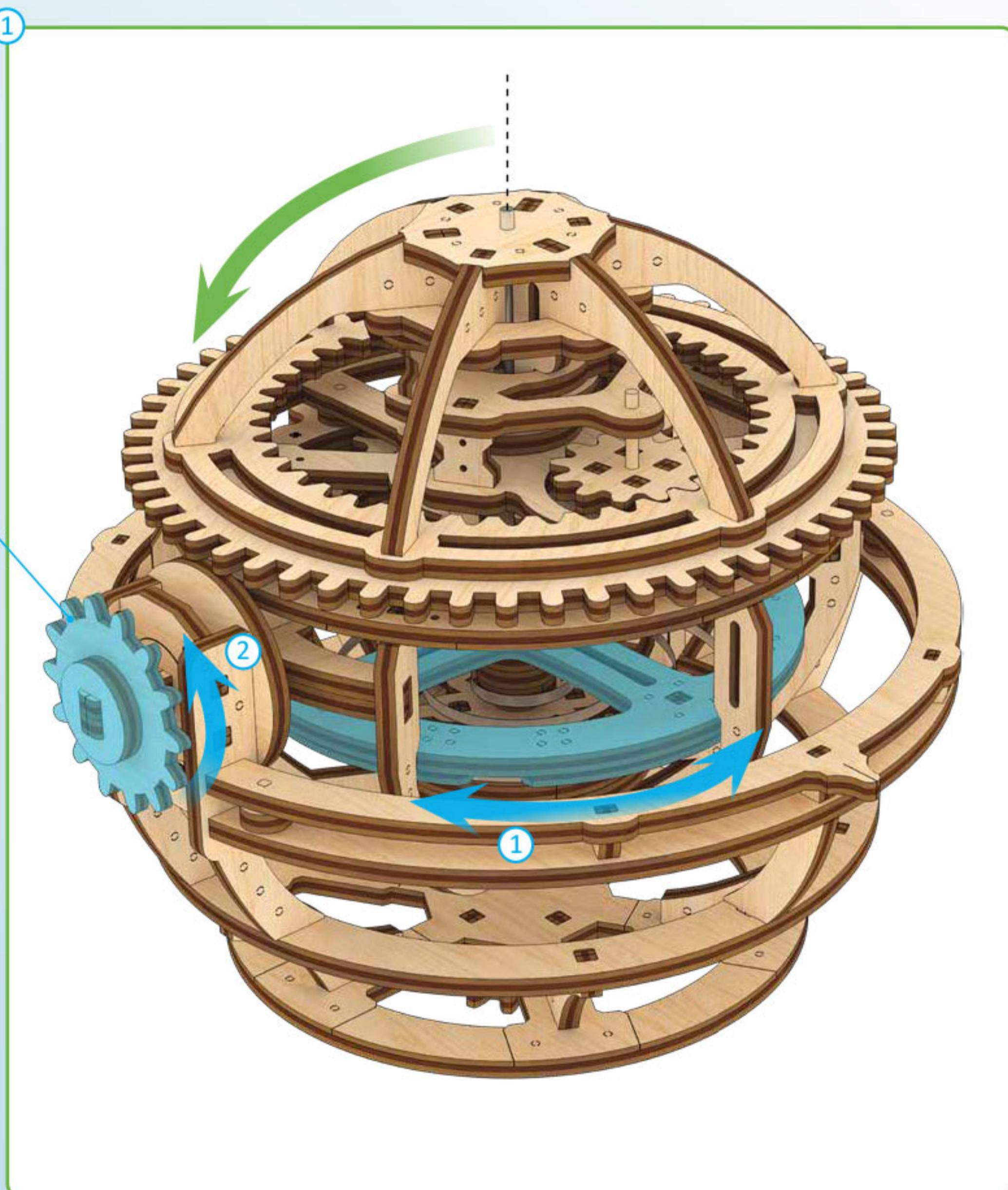
**ENG** Turn lever A (item 2) on the tourbillon, ensure that the tip of the escape wheel tooth falls on the impulse pad of the escape fork in both positions. The easiest way to achieve this is to place the tip of the escape wheel tooth in the middle of the impulse pad of the escape fork (items 3, 4).
